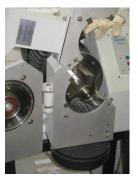
Retsch Power Cutting Mill SM2000 695 r.p.m. / Screen 10mm
