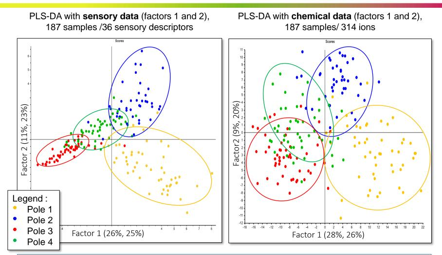
The produced "chemical maps" showed that the headspace PTR-MS analyses of the chocolates allowed retrieving the classification of the 187 samples into the four sensory categories previously determined
