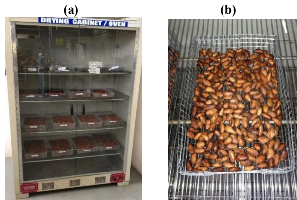
Figure 3. Oven drying of fermented cocoa beans a) Cabinet oven b) Arrangement of cocoa beans on wire tray
